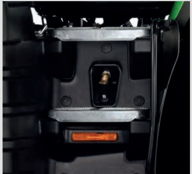
↑ Air supply port and entrance light switch protected under the steps.
