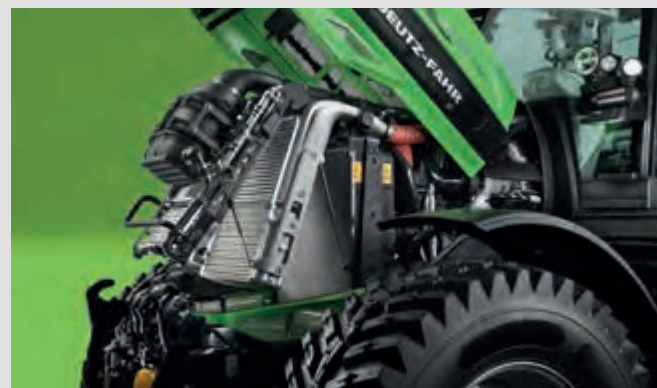
Aluminium cooling system of 6210 and 6230 with one-hand access lever and Powercore air filter with optional cyclone pre-cleaning system.
