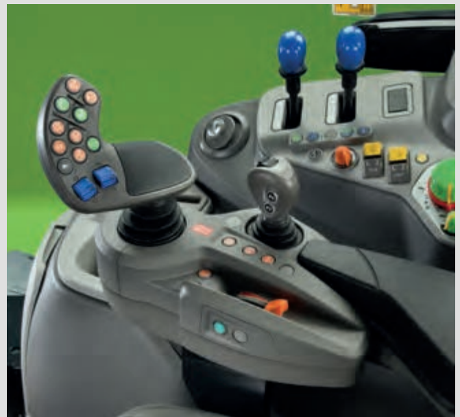
↑ Thumbwheels on the MaxCom joystick and two mechanical levers control the rear spool valves, while the cross lever might be used to control the front loader.
