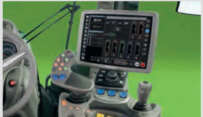
↑ Electric spool valves with comfortable electronic control elements.
