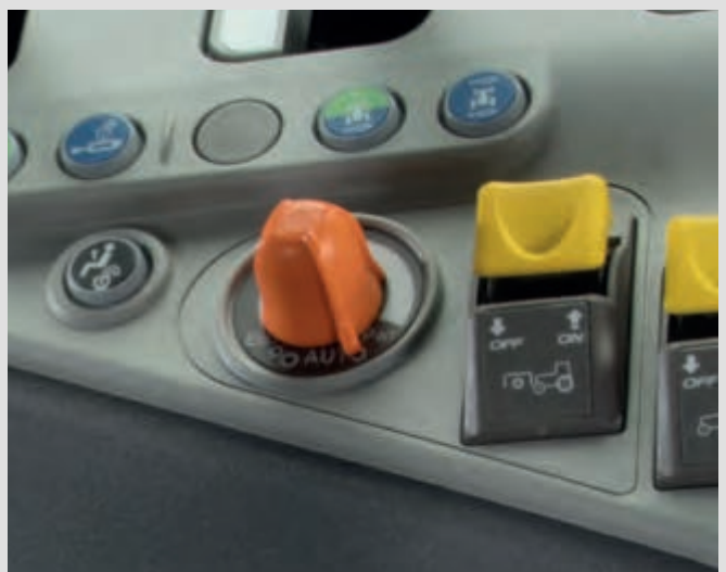
↑ Easy and intuitive – with the Eco/Power adjustment knob the operator can change the APS (Automatic PowerShift) shifting behaviour.
