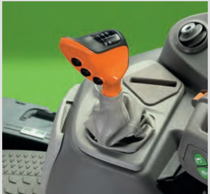
↑ Ergonomic gear lever with ComfortClutch, APS and Powershift buttons.
