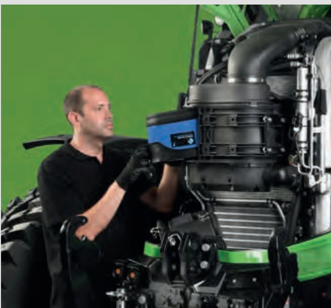
↑ Easy access to the PowerCore air filter.
