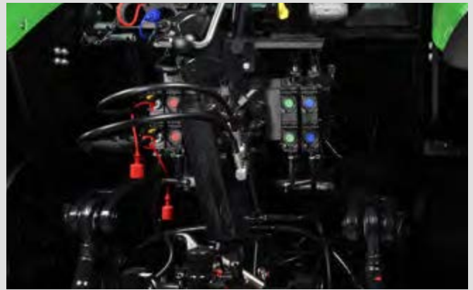
↑ High comfort combined with ease of use: mixed hydraulic configuration with two electric and two mechanical distributors.
