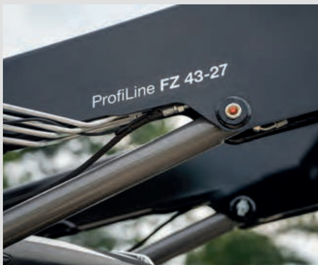
↑ The new ProfiLine front loaders integrate all the hydraulic lines inside the beam rail to ensure they are well protected and the driver has a clear view.
