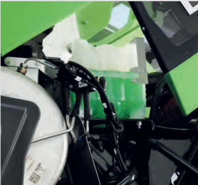
↑ Water tank with steel level marker.
