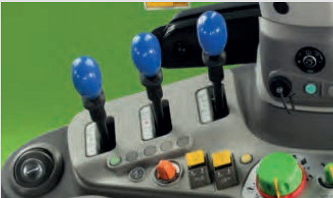
↑ Up to 4 mechanic spool valves with ergonomic single lever controls.
