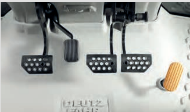
↑ Ergonomic engine brake activation via foot pedal.
