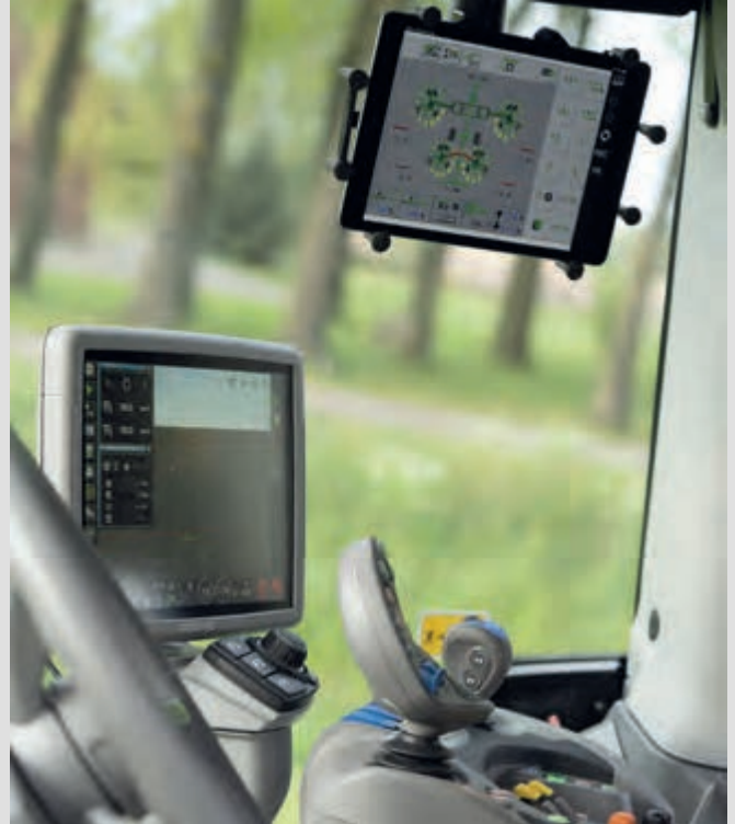
↑ The XTEND function allows the display of SDF Guidance or let you control an ISOBUS implement on an external device, e.g. a tablet.
