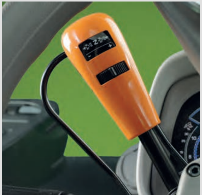
↑ Ergonomic PowerShuttle lever with SenseClutch adjustment dial.
