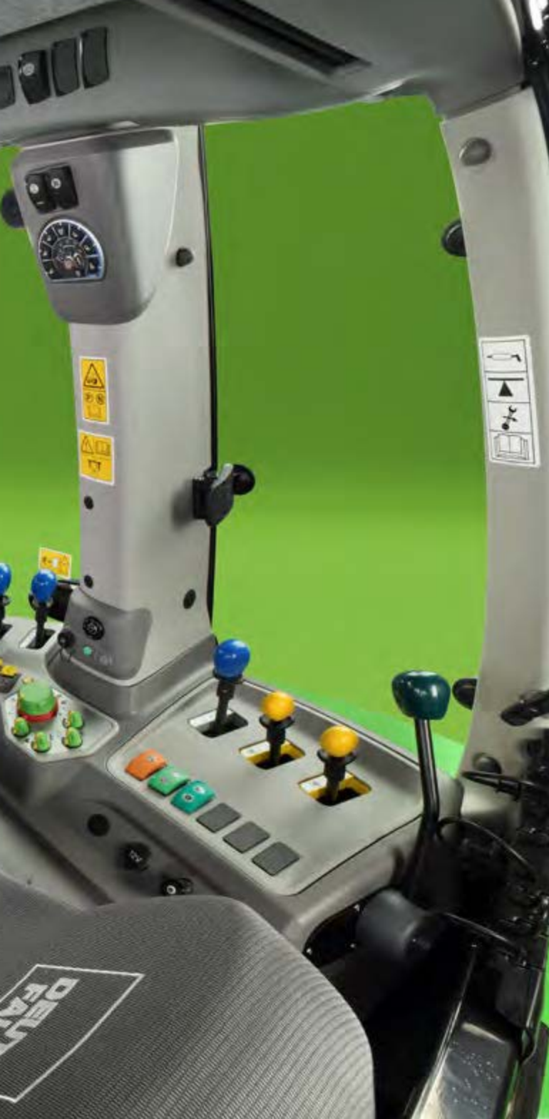
↑ MaxiVision cab equipment with full mechanical rear spool valves is available for Powershift (large picture) and RCshift (picture above) models.
