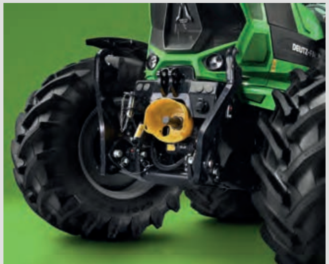
↑ Efficient front lift with up to 3800 kg lifting capacity and optional 1000 front PTO.
