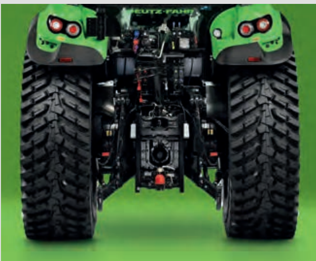
↑ Rear linkage with up to 9700 kg lifting capacity.
